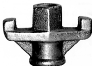
Wing Nut D 15 With two wings, forged thread. Hot-dip galvanized. SW 26, quality : GTW 45, allow. load 90 kN (DIN 18126), weight : 0.33 kg
