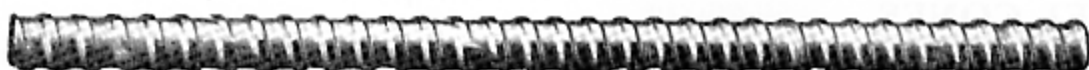
Steel Tie Rod, 15 mm \phi fully threaded, weldable, flexible, allow. load 85 kN, breaking load 170 kN. d max 17 mm, d min 15 mm
