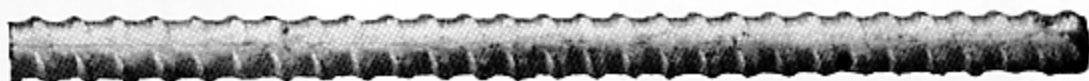
Steel Tie Rod, Dywidag 15 mm \phi quality : ST 885/1080, allow. load 90 kN (DIN 18126), breaking load 190 kN. d max 17 mm, d min 15mm
